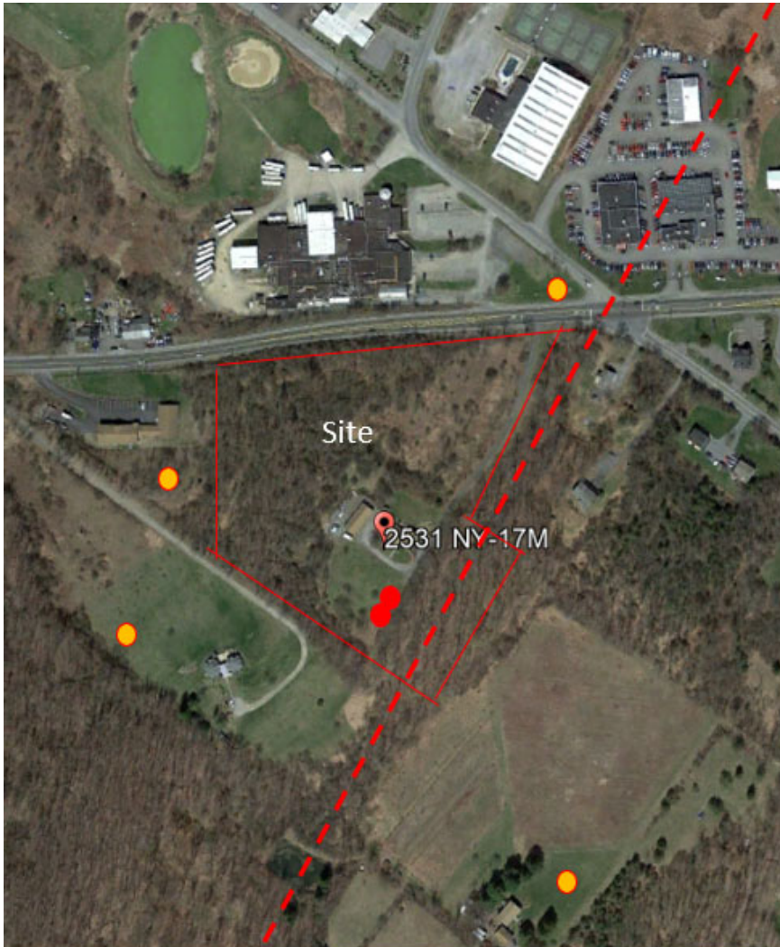
Map 3 – This unscaled map shows the approximate site boundaries, the two wells proposed for capacity testing (red dots), and the approximate locations of off-site domestic wells proposed for monitoring (yellow dots). All locations are approximate. North is to page top. The parcel ID numbers for the off-site wells are listed on the attached site map. The northern most well proposed for monitoring lies approximately along the trace of the dominant linear feature (fracture trace) passing the site.
